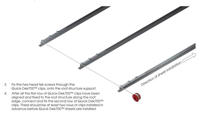
Fix first row of clips with 3 x hex head screws on each clip
