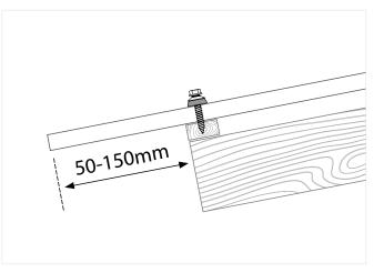
• NOTE: if you plan to install a gutter, use a 50mm overhang.
