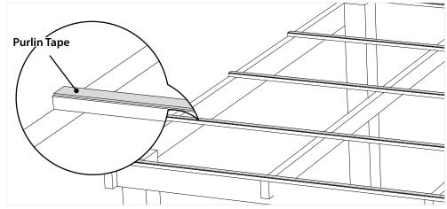
• Applying foam tape on each purlin will reduce friction and noise caused by thermal expansion.
