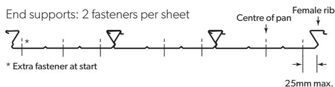
Depending on support spacings used, FLATDEK® can be installed as either:
