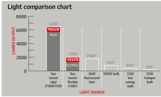
Light transmittance of VELUX Sun Tunnels depends on parameters such as sky conditions (cloudy/sunny), direction of sunlight, orientation and length of Sun Tunnel. VELUX Sun Tunnels in this chart have been tested with a 1 metre shaft, on a 15° roof pitch in summer, at noon on a sunny day using a photometer. (TWR rigid tunnel emits 440 lumens when measured on a cloudy
