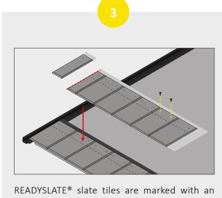
overlapping line to ensure can be accurately laid with ease.
