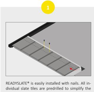
installation process. Once fitted, peel back the protective film.
