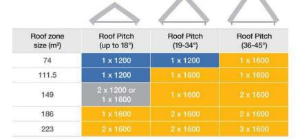
Recommended air intake venting (eaves or soffits) size requirements:
