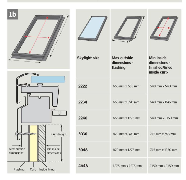
Build curb according to measurements in the chart. Curb height and attachment should comply with building codes and regulations and be secure enough to transfer the skylight loads to the framing members.
