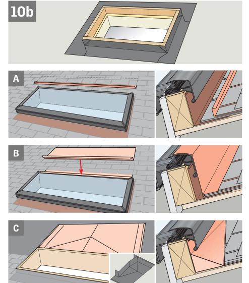
If custom-made flashing is used, consider options  ${\bf A}$ ,  ${\bf B}$  or  ${\bf C}$ .
