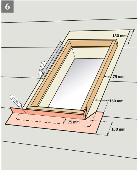
Skylight curbs should be completely wrapped in self-adhesive membrane to ensure waterproofing. To achieve this waterproofing, consider using VELUX roofing underlayment ZOZ 216 (225 mm wide).
