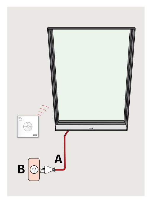
A junction box or an outlet box (not provided with skylight) is required for permanent connection of the 2 m skylight power cable.
