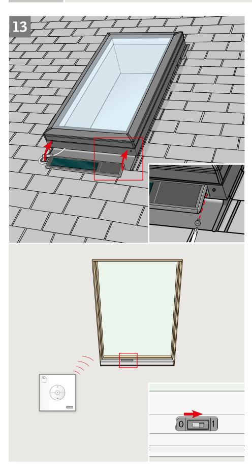
Install solar panel as shown and secure with screws.
