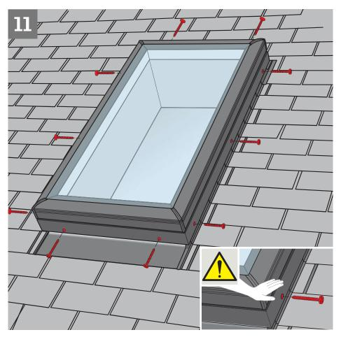
Center the skylight on top of the curb and secure with 45 mm pan head stainless steel screws provided. Screws will penetrate the curb by at least 19 mm.
