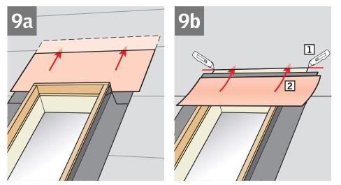
To allow for proper drainage, interweave felt with additional standard roofing underlayment as shown in a for new construction applications.
