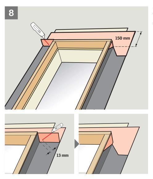
Consider wrapping the curb at top frame of skylight with VELUX roofing underlayment ZOZ 216 and create proper watershedding lap.
