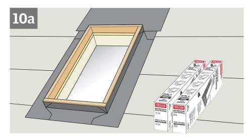
For thin roofing materials, use flashing ECL. ECL is designed for roof pitches 10°-60°.
