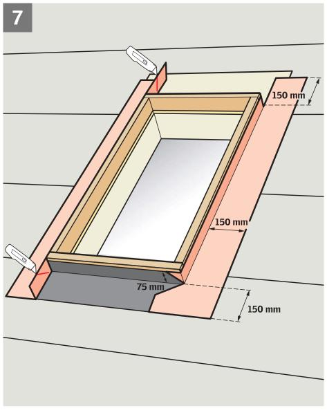
Consider wrapping the curb with VELUX roofing underlayment ZOZ 216 and create water-shedding laps over felt at bottom and sides of skylight 6, 7.
