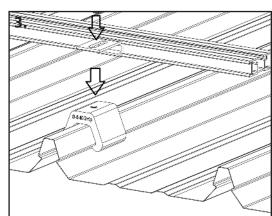
**4. Repeat the above procedure for the second Strut:** You may wish to leave the bolts finger tight, so final adjustments can be made as the condenser unit is mounted to the struts. **(Fig. 4).**
