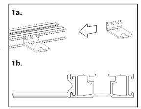
2. Fasten the upslope GRIPPERFIX Strut to the roof ribs:
