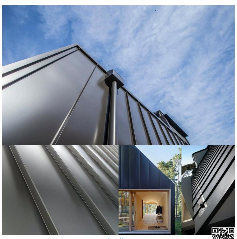
**Snap Lock** is a lightweight cladding system ideal for both roof and wall applications in commercial, industrial and residential environments. Its thin distinctive ribs and wide pans give it visual appeal. Snap Lock looks similar to Standing seam without the need of crimping the joints due to the "snapping" process. Available in 25mm and 38mm ribs, Snap Lock can be manufactured in various widths to suit new construction or renovation projects.
