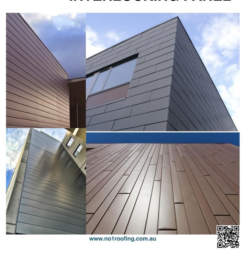
**Interlocking Panel** is a contemporary looking wall cladding system installed with a ventilated air gap for external and internal applications. The panels are connected by an interlocking groove giving it an elegant appearance of a recessed joint. The reveal panel can range from 185mm to 385mm in width and lengths up to 6.0m. Shadow lines can range from 0mm to 25mm.
