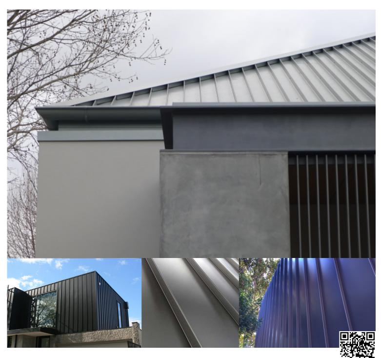
**Nail strip** can be used for vertical facade or roofing applications. Available in 25mm and 38mm rib height, it comes in various widths and lengths to suit your project. The Nail Strip panel has a thin rib and wide tray with a perforated fixing strip along one side. There is no need for fixing clips and the additional operation of seaming. This ensures speed and ease of installing panels whilst allowing for expansion and contraction.
